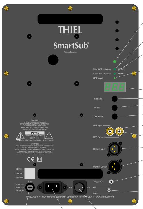
This light and the one on the front of the subwoofer will glow green if the amplifier is currently operational, and red for 5 seconds during start-up or if the amplifier is set for auto-on that is not currently activated. It will flash in various colors and patterns when heat or line voltage is a problem.
